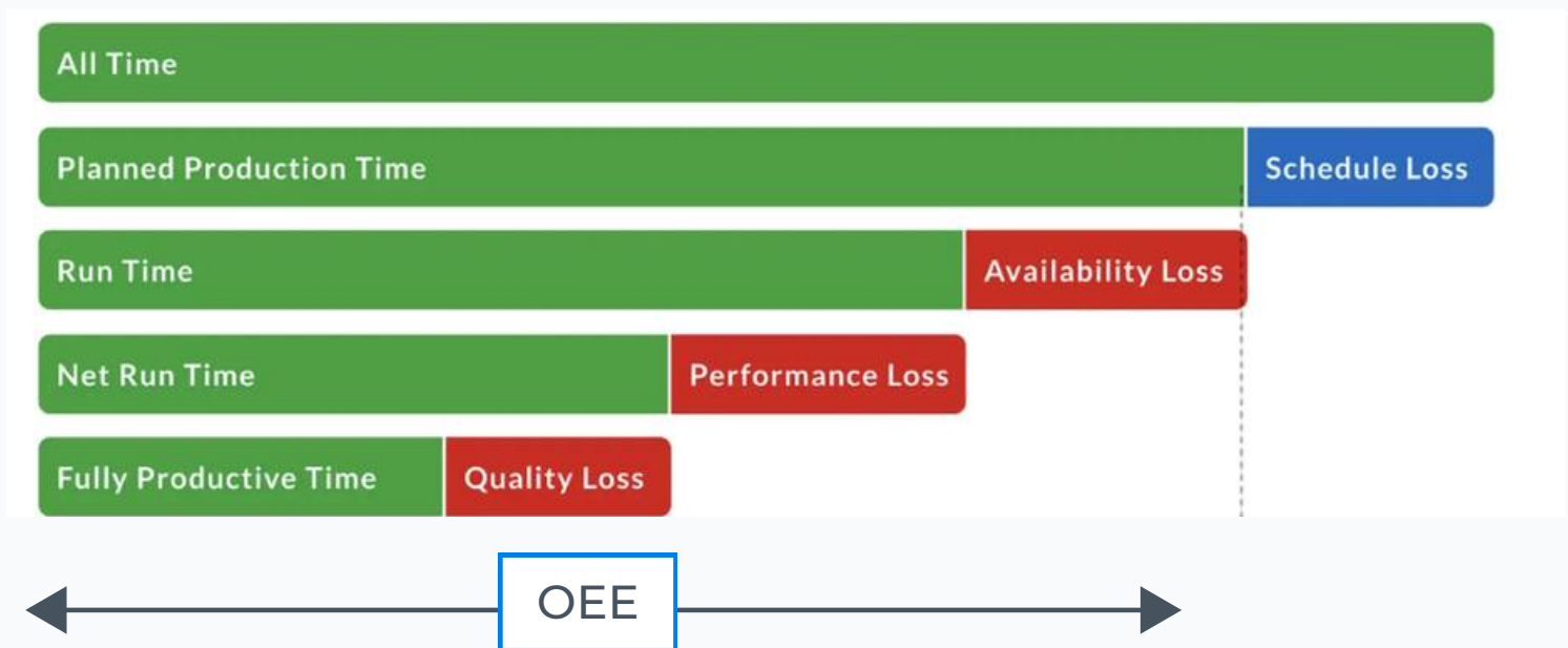
Image 2: OEE measurement and its losses.
